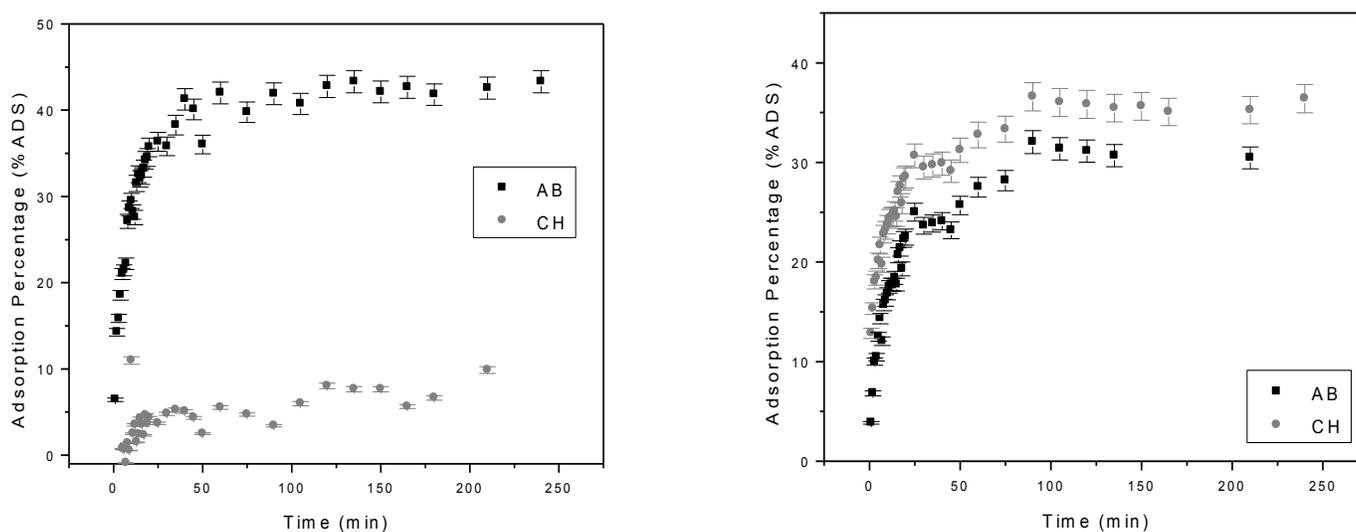
**Figure 8:** Time-dependence of the adsorption of En (left) and Pe (right) onto AB and CH.
