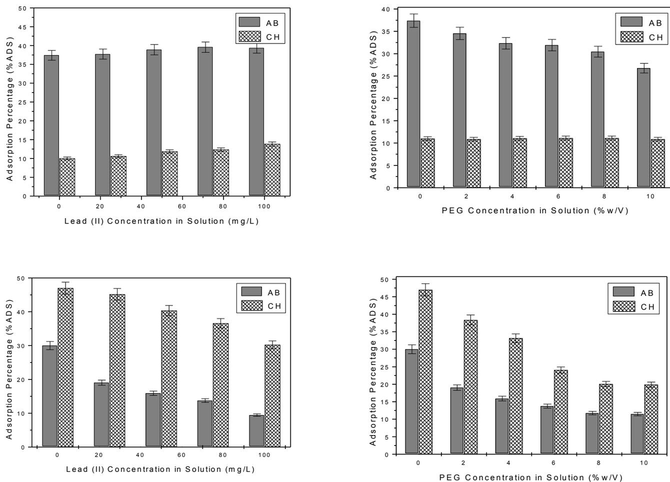
**Figure 7.** Effect on metal ions on the adsorption of En (top left) and PE (top right) and PEG on the adsorption of En (bottom left) and Pe (bottom right).
